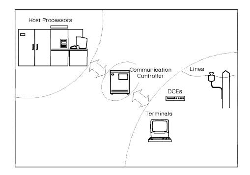
In today's communication networks, the communication controllers save much data processing power by handling sophisticated functions to control the data flow between host processors and the network of terminals.
