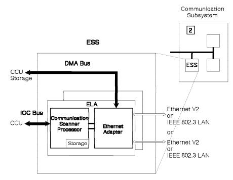
The ESS consists of up to two Ethernet LAN adapters (ELAs).
