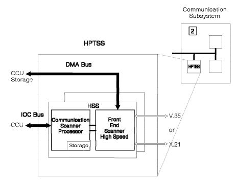
The HPTSS consists of up to two high-speed scanners (HSSs).
